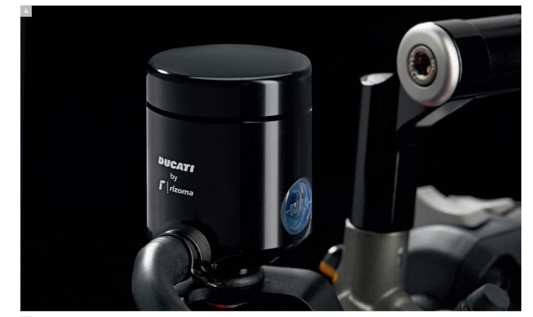
4 Brake fluid reservoir - Clutch fluid reservoir
